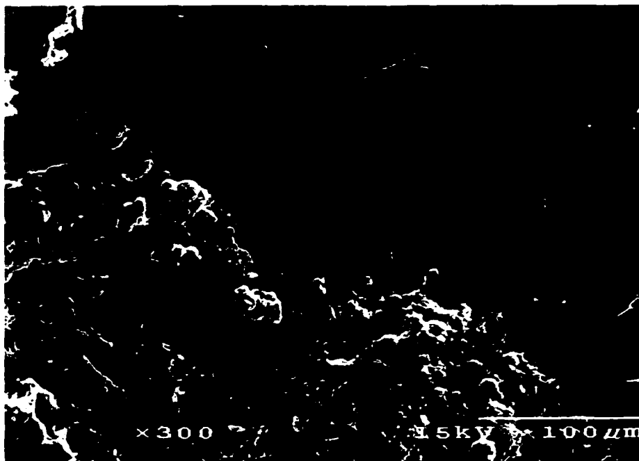
Figure 8. Tightly bound interface of composite material at sheared surface of embedded sand grain.
